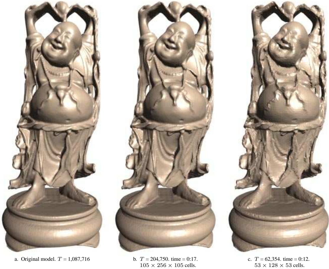
Figure 5.1: Out-of-core simplifications of Buddha model. The number of triangles T , the simplification time (minutes:seconds), and the number of cluster grid cells are indicated.
