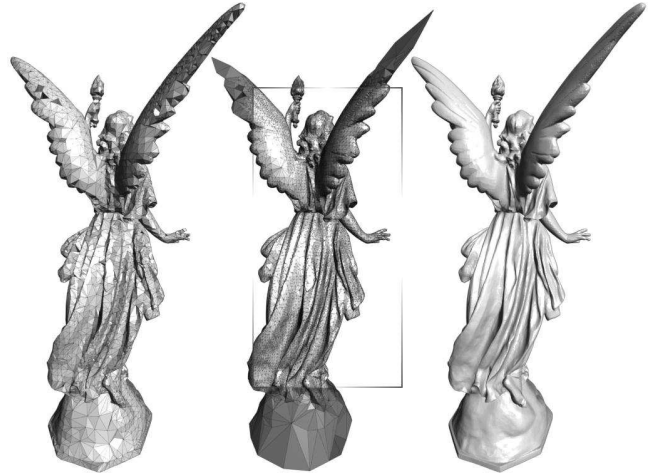
Figure 1: Various view-dependent meshes produced by our system. The mesh in the middle has been coarsened aggressively outside the view frustum (here shown as a rectangle).
