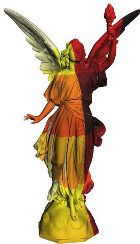
Figure 1: Illustrations of the coherence in the layout of a mesh: On the left the original layout; on the right the layout after reordering the vertex and triangle arrays using spectral sequencing. The large rendering color-codes triangles based on their position in the array. The layout diagram connects triangles that share the same vertex with horizontal line segments (green) and vertices referenced by the same triangle with vertical line segments (gray).
