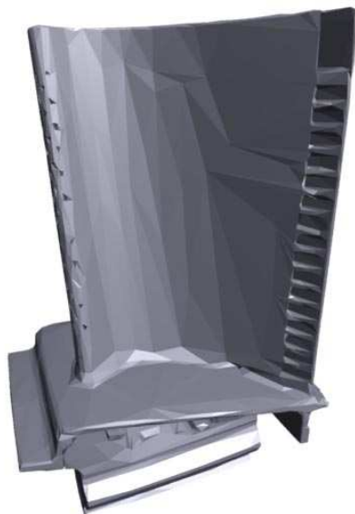
3d. Image-driven simplification using front-face culling in 10 of 20 views. T = 8,191 . time = 1:33:34. d_{RMS} = 2.10 .
