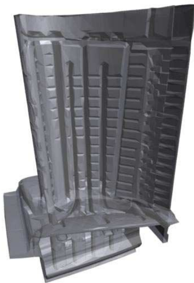
3a. Geometry-driven simplification. T = 8,191 . time = 27:06. d_{RMS} = 2.16 .
