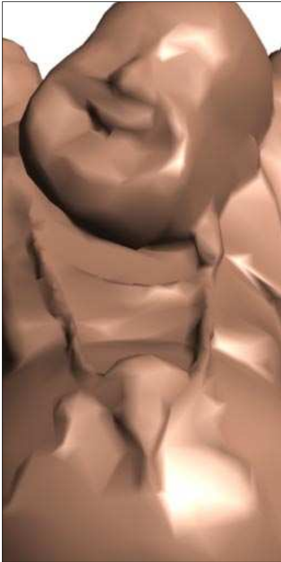
9a. Closeup of Gouraud shaded model optimized for flat shading.
