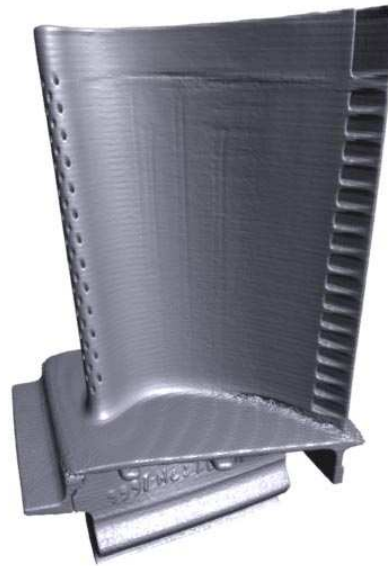
2b. Original turbine blade model. T = 1,765,388 .
