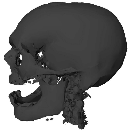
Figure 13: Approximation up to the size of one and a half pixel. The original dataset is reduced from 811k vertices (=1622k triangles) to 22.7k vertices (47.1k triangles). This is a reduction rate of 97.2 %.
