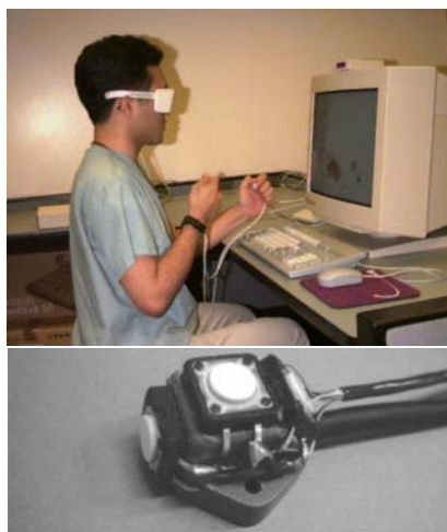
Figure 1: (a) A user using the two-handed stereo interface to SFA.(b) A 3D tracker with buttons attached.
